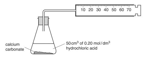
The diagram below shows the gas syringe containing the volume of carbon dioxide collected in one minute.
